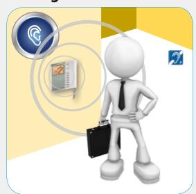
So that hearing aid wearers can perfectly hear everything said by a visitor speaking into the external unit, Comelit technology features a Magnetic Induction system (T-COIL): this function enables transmission of audio signals from the internal unit to the hearing aid and amplifies voice communication (T-COIL).
