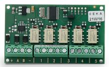
auxi relay has 5 relay outputs (1A) which may be used for manage all kind of loads in lares 4.0 Control Panel series.
