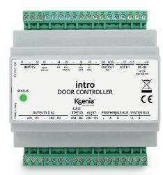
intro door controller module is a BUS peripheral that can be connected to the lares 4.0 control panel, it is completely developed by Ksenia, from design to final production, in Italy.
